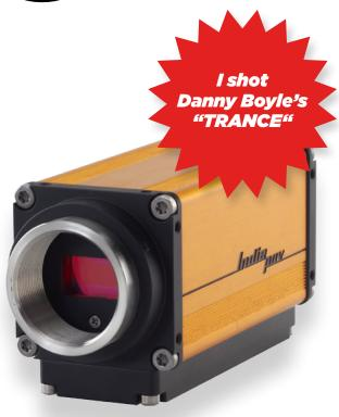
The IndiePOV is a miniature HD camera with breathtaking features. It incorporates a 2/3 inch CMOS imager and delivers 1080p high definition at up to 30 frames per second in 10 bit uncompressed 4:2:2 and 12 bit RAW. It operates stand-alone without the need of a control-box.
